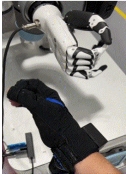
Fig. 4.10: Human and robot hand motion mapping.
