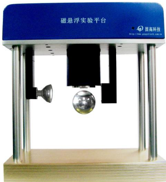
Figure 4.32 Photograph of the magnetic levitation experimental equipment
