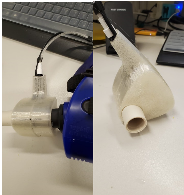
Figure 5.4 The first fused deposition iteration of the waterproof housing
