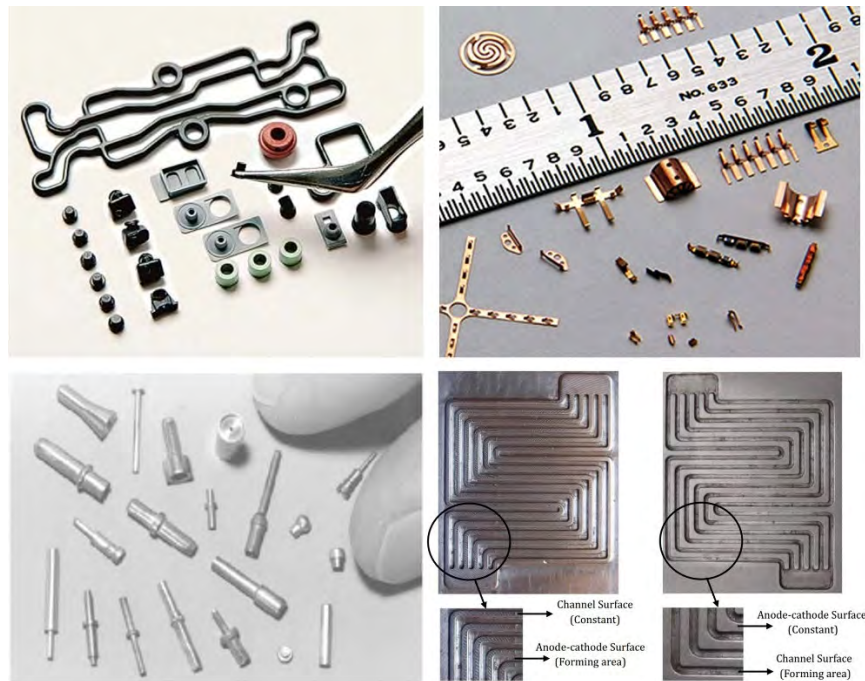
Fig. 2.1 Meso/micro-scaled components and structures fabricated by forming processes [3, 34-36].
