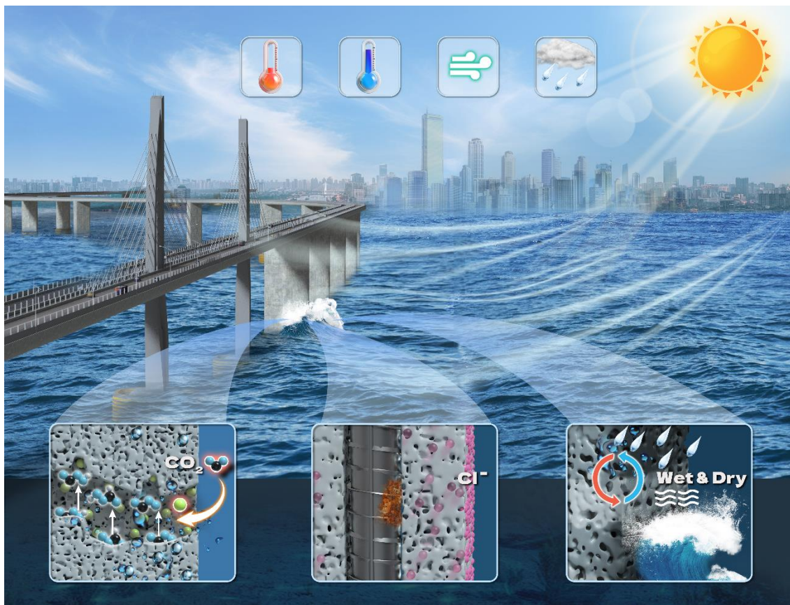
Figure 2.1. Schematic of different exposure zones in a coastal RC structure and the critical micro-climate factors affecting chloride transport and chloride threshold in each zone.
