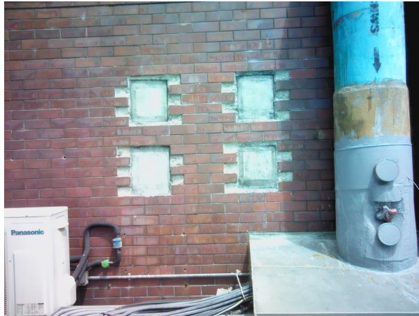
Figure 6.22: Embedded defects and the marks on the sample wall at PolyU Position B.
