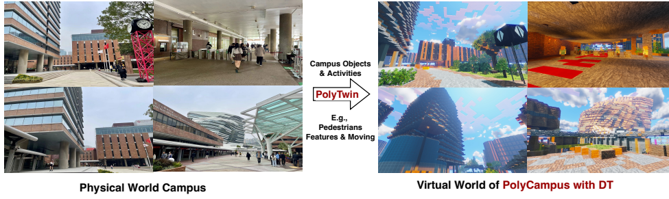
Figure 3.7: PolyCampus Prototype: Real-world campus activities (pedestrian movements and attributes) are captured by edge AI and projected as digital twins into a virtual campus, enhancing immersion for metaverse users.
