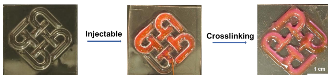
Figure 4.18 The injectability of host-guest hydrogel.
