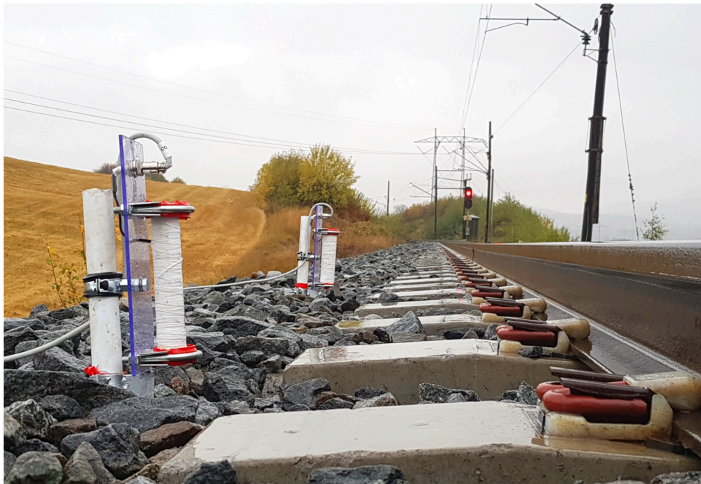
Fig. 1-13 In-situ experimentation of the magnetic field energy harvester developed in [71].
