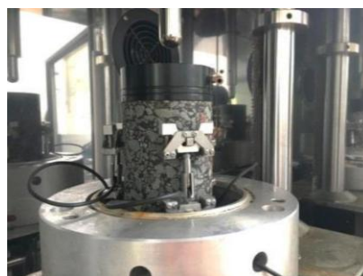
(b) Uniaxial compressive dynamic modulus test
