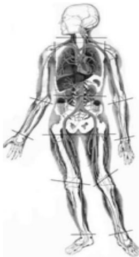
Figure 2.6. Schematic illustration of the human segmentation used in Huizenga's thermophysiological model. (Huizenga, Zhang, & Arens, 2001).
