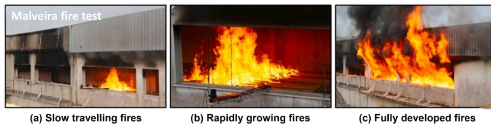
Fig. 4.1. Diagram of travelling fire behaviour in Malveira fire test [30]: (a) Slow travelling fires; (b) Rapidly growing fires; (3) Fully developed fires.
