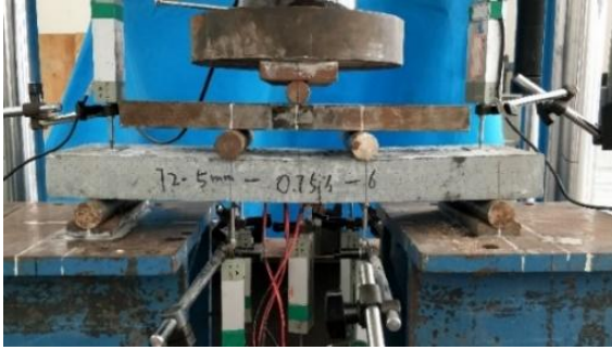
(d1) Thin plate four point bending test
