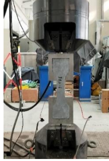
(c1) Dog bone tensile test
