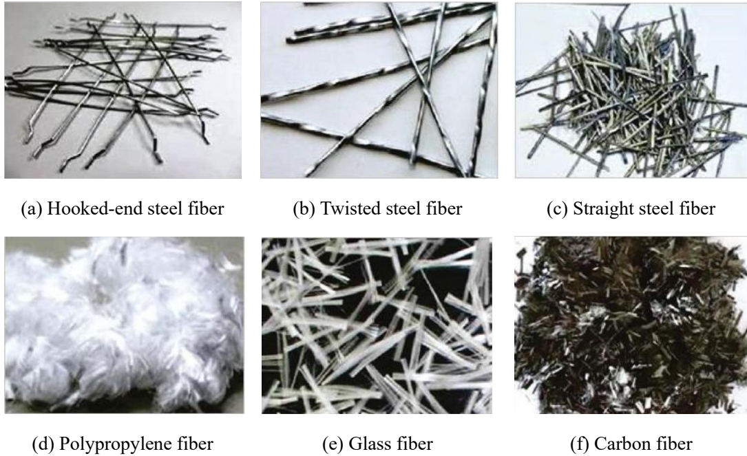
Figure 2.8 Different types of fibers used in UHPC [79] .
