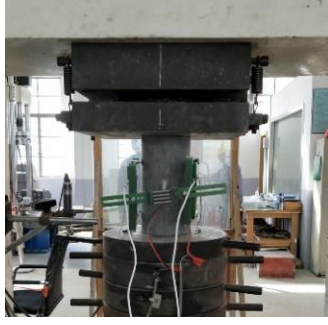
(b1) Cylinder modulus test
