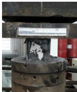
(a1) Cubic compression test
