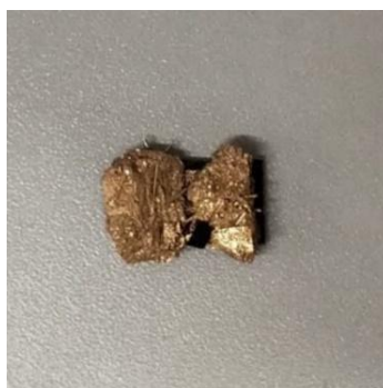
Figure 3.7 Gold plating treatment on the surface of the sample.
