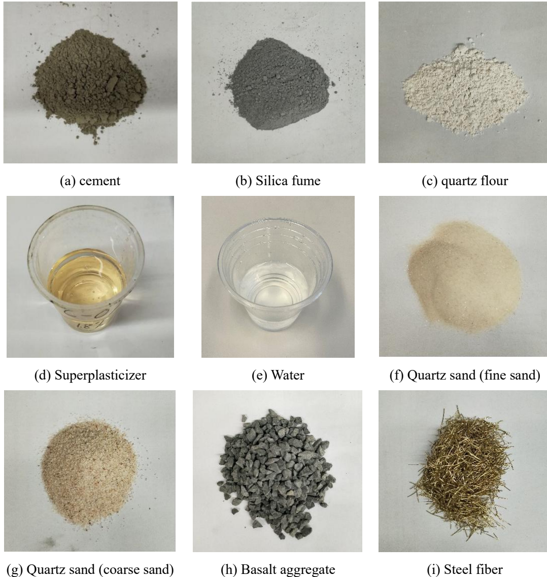
Figure 3.1 UHPC raw material.
