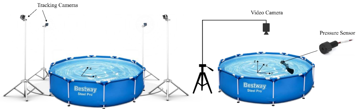
Fig. 5.18: Left : Setup for on-surface 2D tracking. Right : Setup for underwater tracking.
