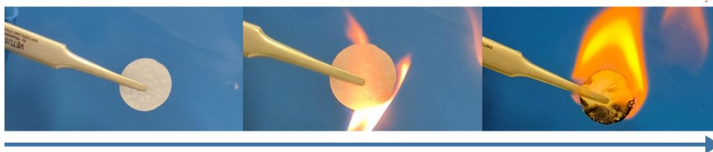
Figure 3.4 Flammability test of glass fiber membranes soaked with 0.5 M \text{Mg}(\text{TFSI})_2/\text{PC} .
