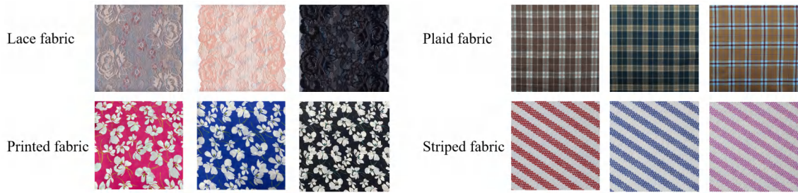
Figure 4.1: Comparison of images with identical patterns across lace, printed, plaid, and striped fabrics reveals that lace fabrics present greater challenges. Unlike other fabrics, lace undergoes not only color changes but also alterations in surface texture characteristics. In contrast, the other fabrics exhibit changes only in color.
