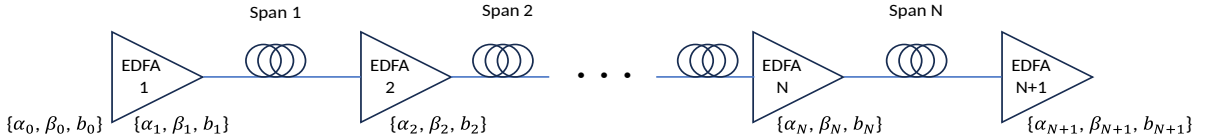
Figure 4.1: Schematic diagram of the transmission link. Gaussian noise is independently added to \lambda and b at each EDFA.
