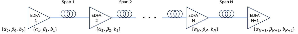
Figure 6.2: Schematic diagram of the transmission link. ASE noise is independently added to \lambda and b at each EDFA.
