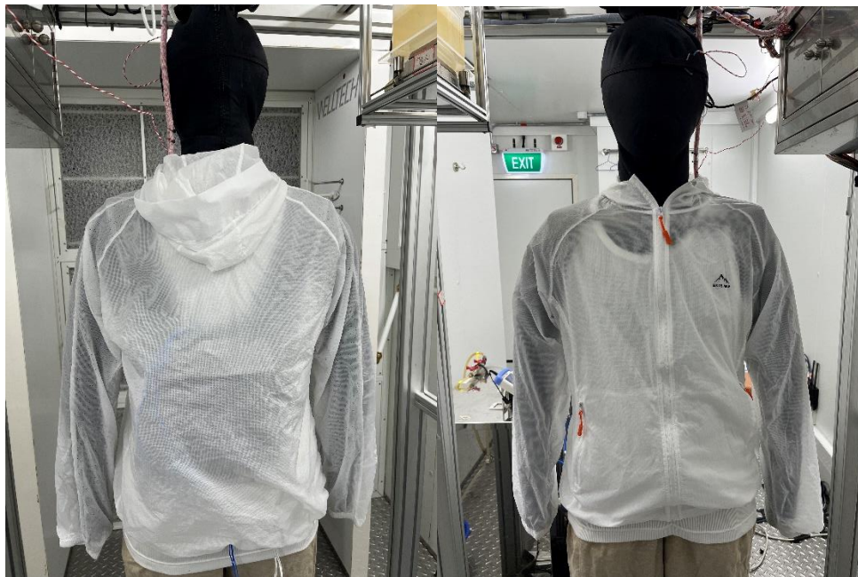
Figure 7. 1 Perspiring thermal manikin-Walter in testing condition.
