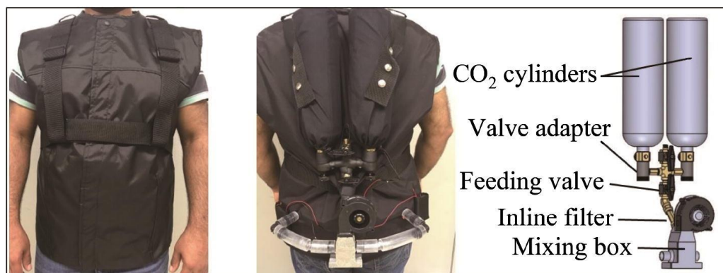
Figure 2.7 Front and back view and the air treatment system of the Air/CO 2 cooling garment.[33]
