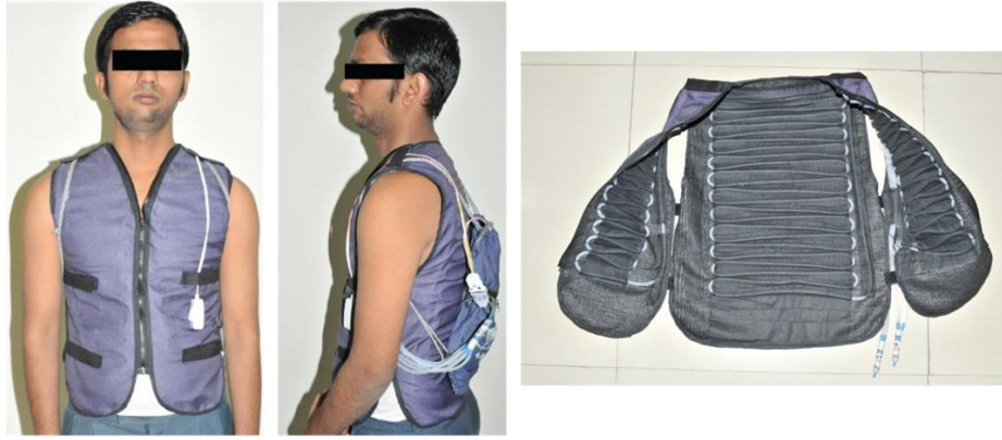
Figure 2.10 Front view and side view of Personal cooling garment with silicon tubing.
