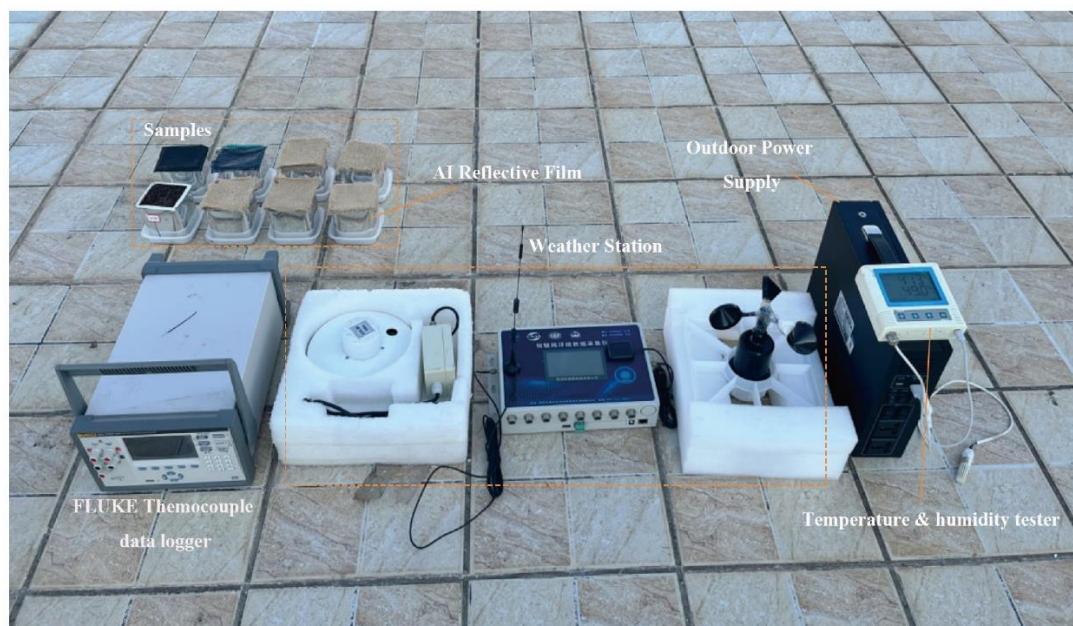
Figure 5-3 A photograph of the experimental setup for temperature change and water retention under sunlight. This setup is mainly consisted by a thermocouple data recorder, a temperature and humidity recorder, and a weather station. The chamber of the soil container is isolated from the surroundings by an Al film to reflect sunlight. The temperatures of soil and fabric surface are real-time measured by thermocouples recorder.
