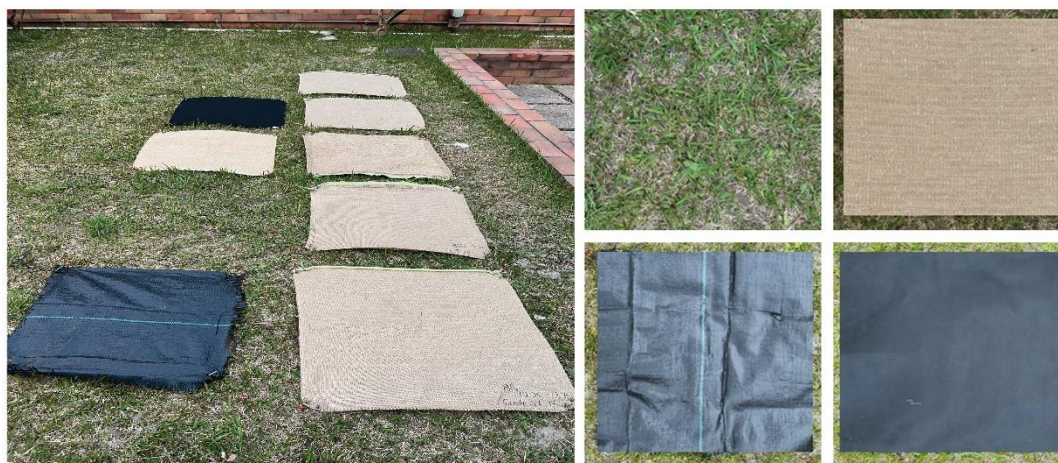
Figure 5-4 Photographs of the outdoor experiment condition to test the weed control of different covering materials. All fabrics of size 500 mm * 500 mm were laid in an outdoor experimental site with adequate sunlight in the campus of Hong Kong Polytechnic University, Hong Kong, China (114.1795 °E, 22.3051 °N).
