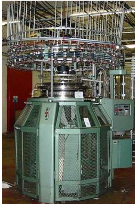
Figure 7-1 Fukuhara FXC-Z/3S multi-feed circular knitting machine (the same type as the machine used in this study)
