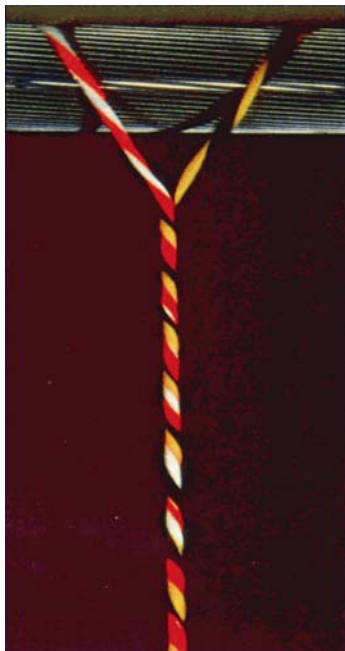
Figure 3-3 The formation of a sirospun yarn (CSIRO textile and fiber technology)
