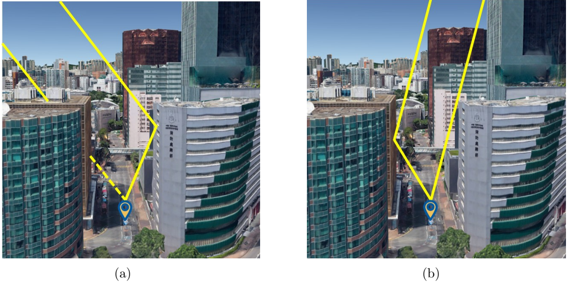
Figure 1.1: Illustration of GNSS NLOS reception and multi-path reception in urban canyons. (a) For NLOS reception, only one reflected signal is received. (b) For multi-path reception, it is a superposition of multiple signal components.
