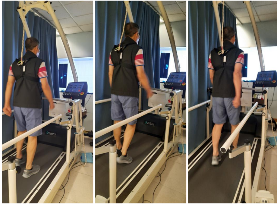
Figure 6-3. Participants walking on a treadmill while wearing the experimental foot orthoses during gait analysis.
