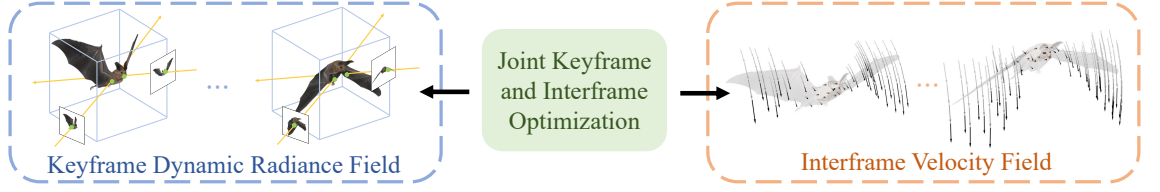
Figure 3.1: The three major components of our framework: Keyframe Dynamic Radiance Field, Interframe Velocity Field, and the Joint Keyframe and Interframe Optimization module.
