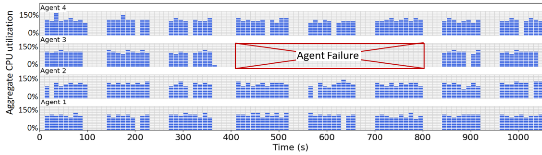
Figure 7.10 Real-time stacked CPU load grid under agent failure and recovery
