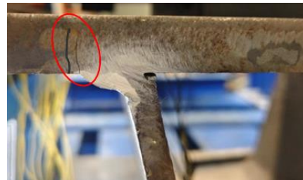
a) Typical fatigue crack of WTD
