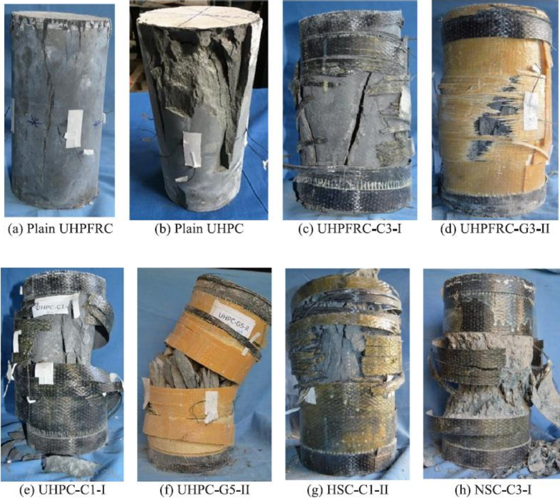
Figure 2.15 Typical failure modes of FRP-confined UHPFRC/UHPC [extracted from Wang et al. (2018)]
