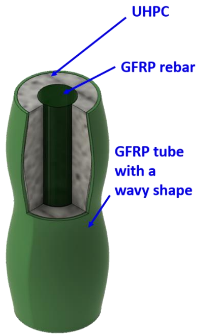
Figure 1.3 Hybrid rebar with a wavy shape
