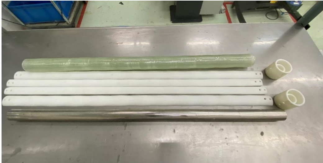
Figure 3.3 3D printed internal mould for filament winding
