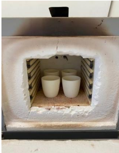
(a) Electric Muffle Furnace
