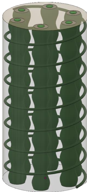
Figure 1.3 Hybrid rebar with a wavy shape
