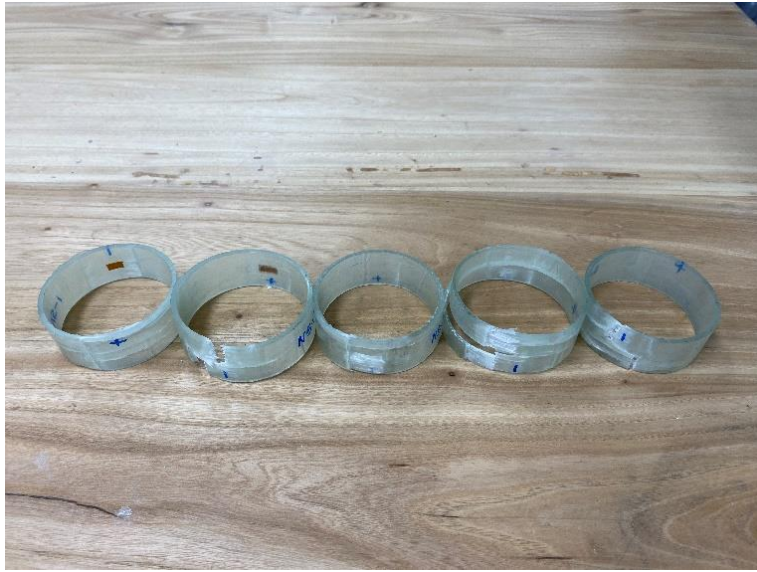
Figure 3.15 Failure modes of specimens in the split disk tests
