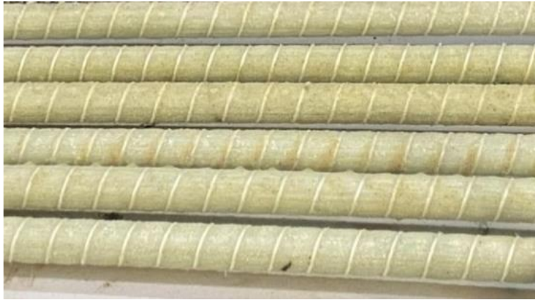
(a) Sand-coated and helically wrapped FRP rebars
