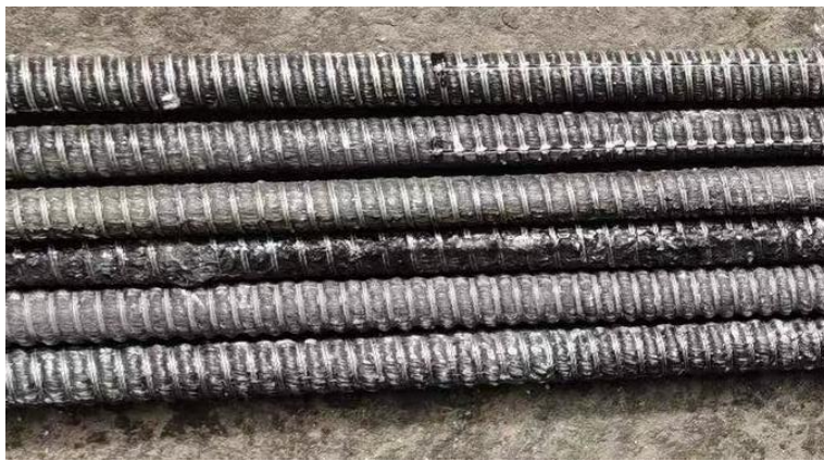
(b) Helically ribbed FRP rebars
