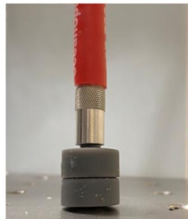
Figure 6-7 3D printed sensor housing
