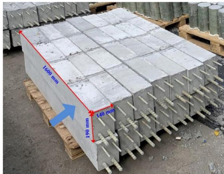
Figure 3-8 FRP reinforced SWSSC beam samples
