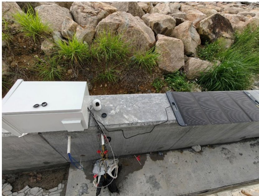
Figure 6-14 The fluorescence-based sensing system for monitoring chloride and sulphate in the outdoor waterproof metal box and solar panel
