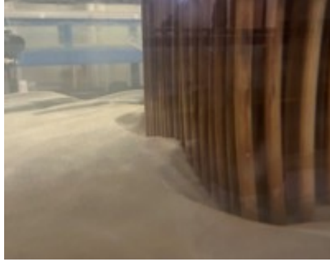
Figure 3.4: Bedform observed upstream of the vegetation array. In this region, the velocity was not affected by the presence of vegetation patch, suggesting that the incoming velocity was below the critical threshold necessary to initiate sediment movement, thereby maintaining a flat bed.
