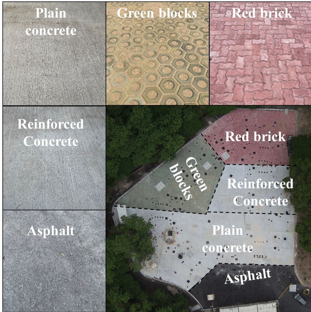
Figure 4-1 Overview of the leakage detection ground showing five different pavement types and corresponding photos
