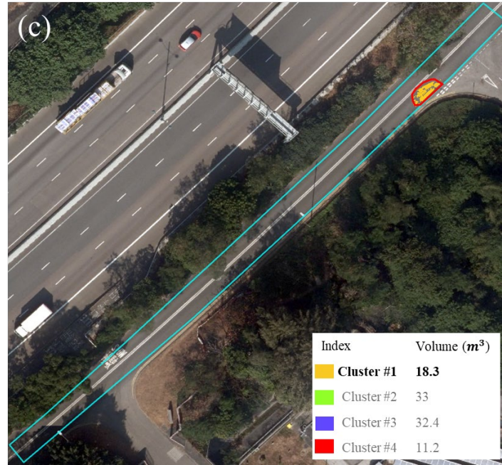
Figure 7-12 Illustration of change clusters identified for Period 2 (a) Change clusters in amplitude difference image slices; (b) Change clusters in IF difference image slices; (c) The intersection of change clusters in amplitude and IF difference images
