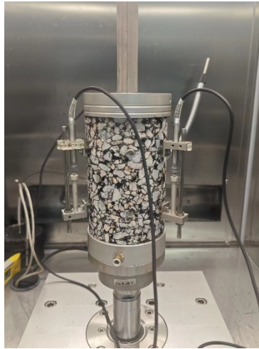
Figure 5.19 Dynamic modulus tests of asphalt mixtures
