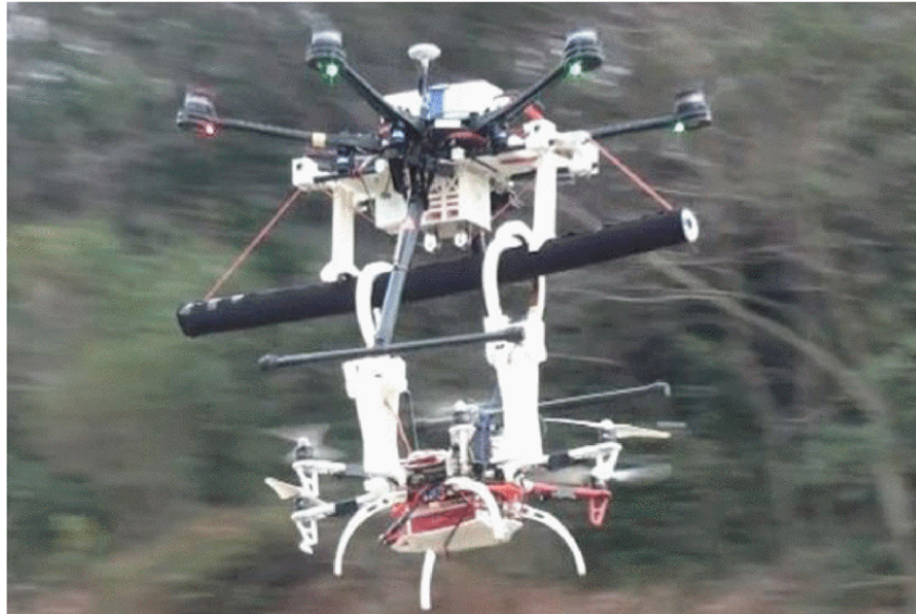
Figure 6: Transportation of working UAV [42]
