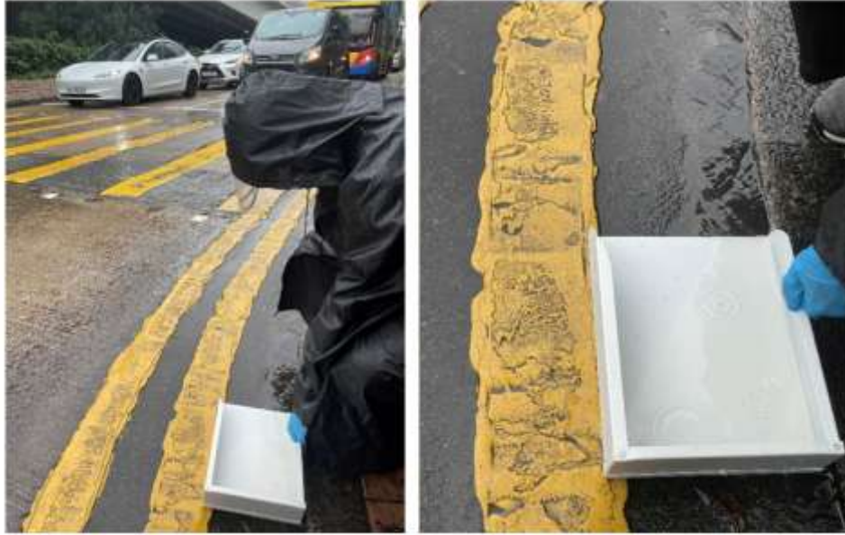
Figure 3.2. Pictures of collecting runoff samples on road surfaces during rainfall using a stainless-steel rain dustpan.
