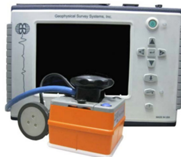
Figure 2.2 GSSI 2GHz palm antenna for laboratory tests
