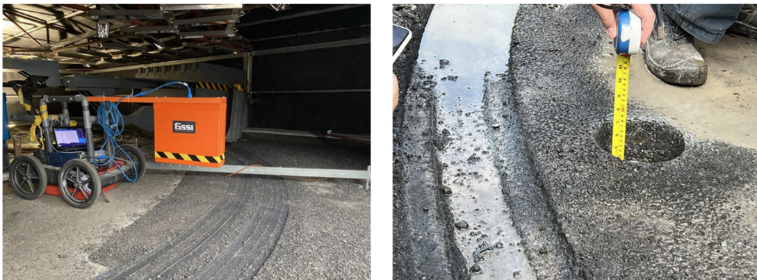
Figure 4.16 Field GPR tests of case II: (a) GPR survey; (b) drilled core samples
