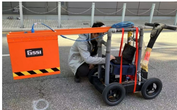
Figure 2.1 GSSI 2GHz air-coupled horn antenna for field surveys
