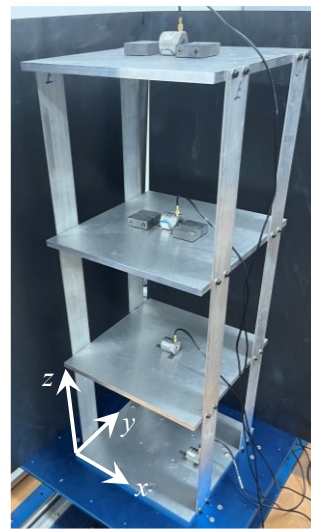
Figure 6.13 Laboratory-tested three-story frame
