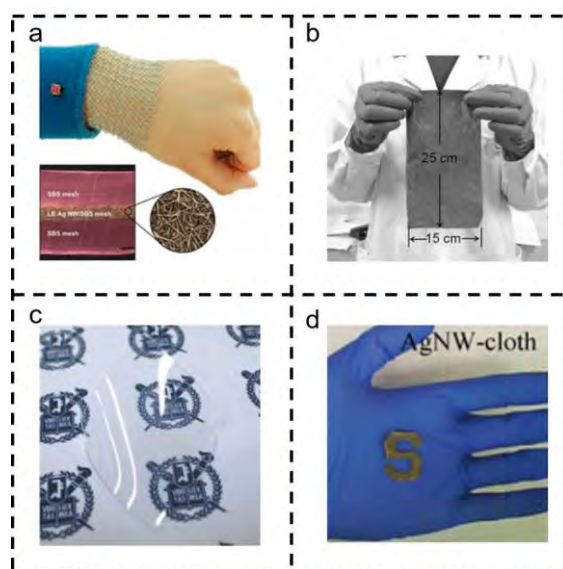
Figure 2.7 Different types of flexible heaters based on the Joule effect. a) Stretchable heater using ligand-exchanged silver nanowire nanocomposite. 71 b) Ultrathin, washable, and large-area graphene papers. 79 c) Highly stretchable and transparent metal nanowire heater. 72 d) metallic nanowire-coated textile. 77
