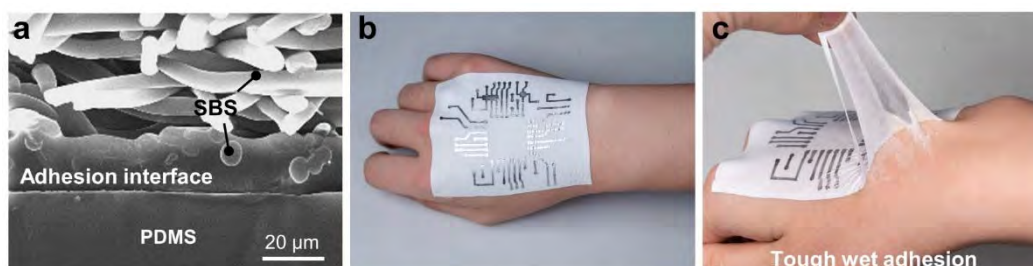
Figure 4.16. a , SEM image showing the adhesion interface of the WADE-skin adhered to a PDMS substrate. b-c , Digital images showing the tough wet adhesion between WADE-skin and human skin; a WADE-skin adhered to the human hand ( b ) and was torn apart by stretching the substrate ( c ).
