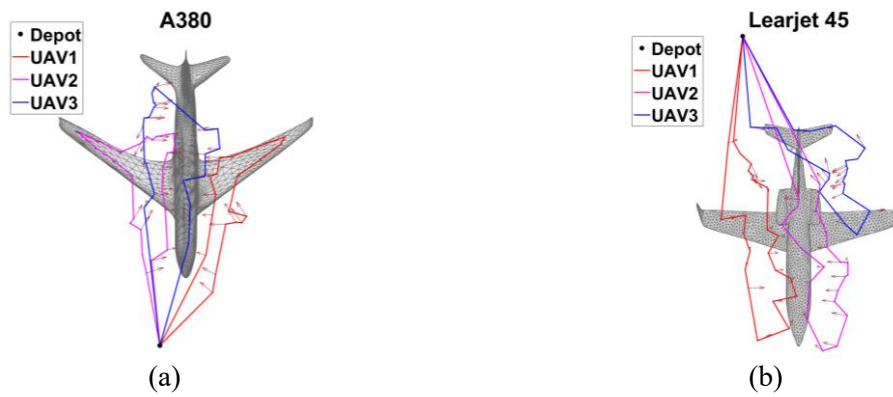
Fig. 5.23 Computed path of the two inspection missions.
