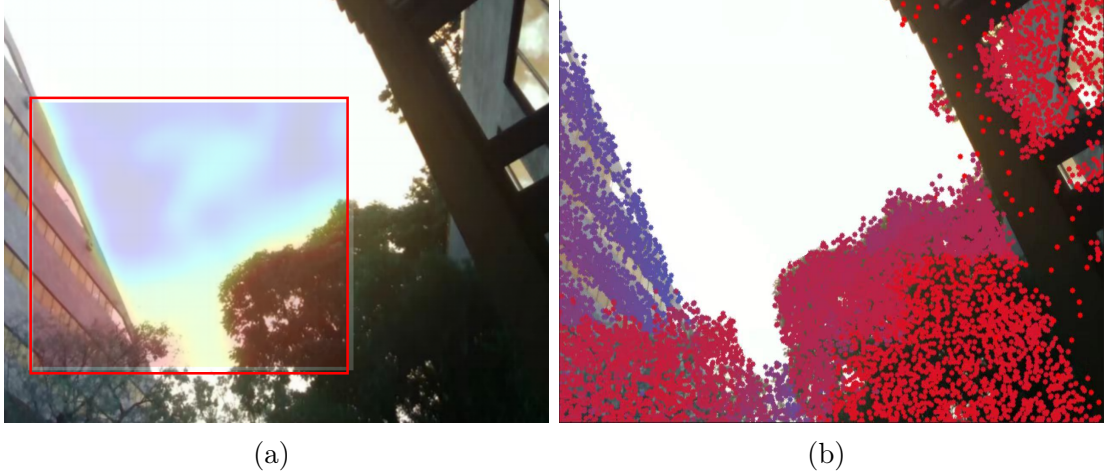
Figure 3.15: Image fusion result of RGB image and LiDAR point cloud. (a) Raw RGB image, the FoV of the thermal camera is shown in the red box. (b) RGB image with LiDAR point cloud projection.
