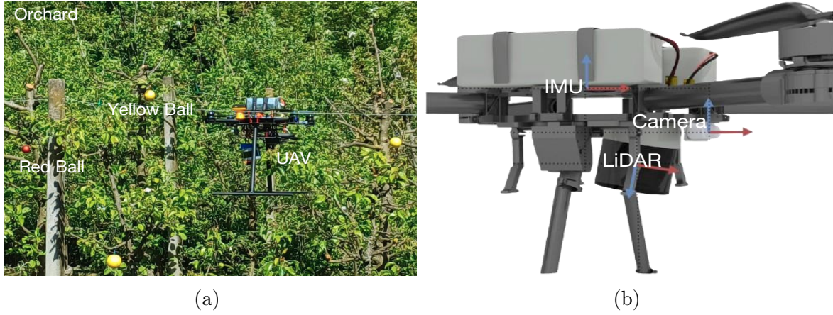
Figure 6.6: ICUAS'24 dataset collection scenario. (a) The dataset collection orchard environment. (b) The UAV configuration.
