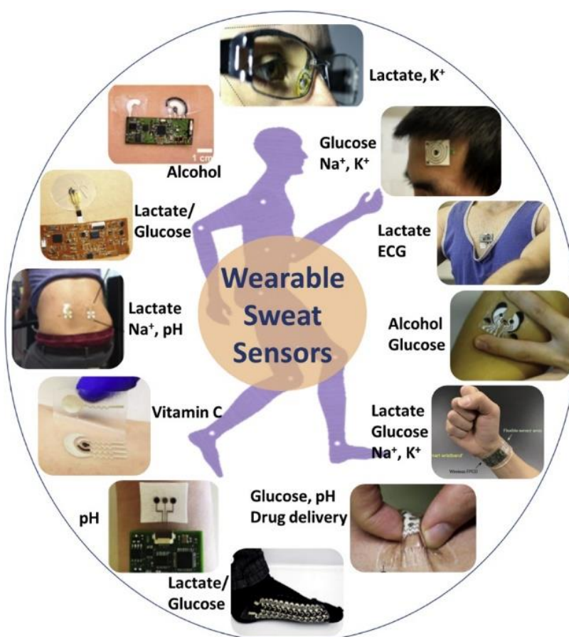
Figure 2.11 Wearable sweat sensors for multiplexed detection of key health-related biomarkers 61 .
