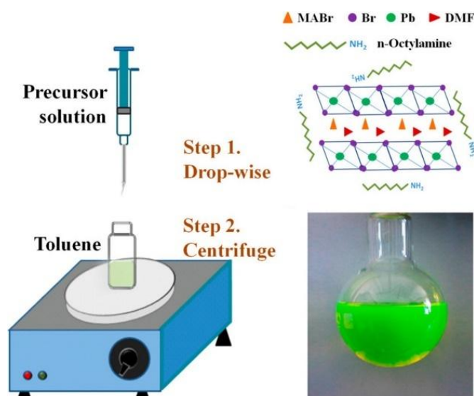
Figure 2.7 Schematic diagram in the synthesis process of \text{CH}_3\text{NH}_3\text{PbBr}_3 QDs using the LARP method. 21
