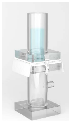
Figure 3.11 The homemade apparatus for hydrostatic pressure test.
