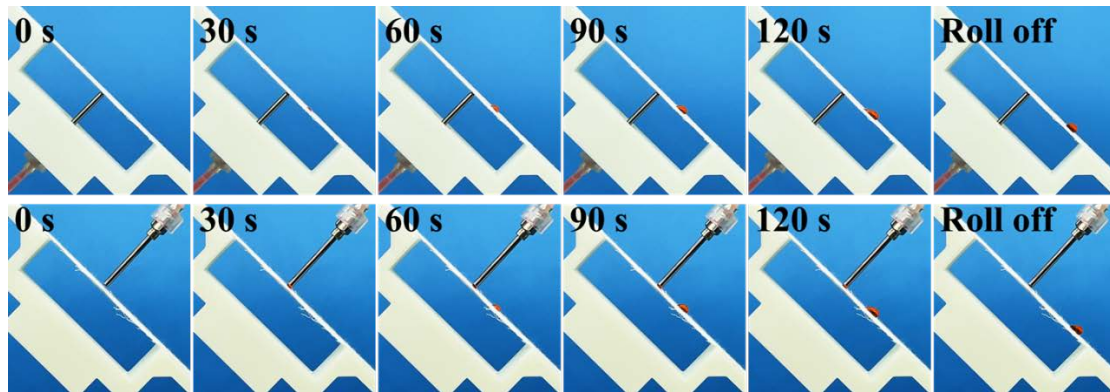
Figure 3.15 The directional liquid transport property of the fabric. The water was dyed red to facilitate visual observation.
