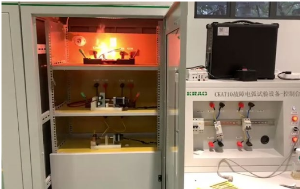
Figure 1.2 Arc faults caused by insulation damage.
