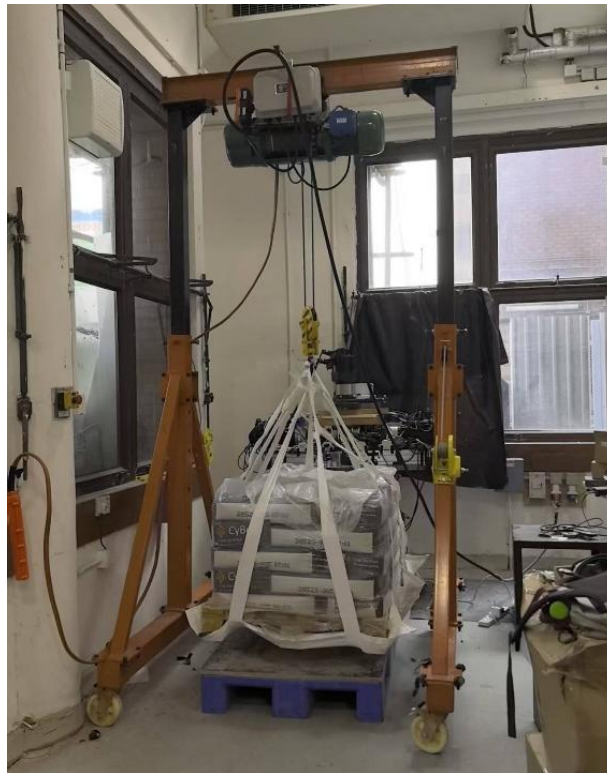
Figure 8-9 Static Load Testing (750kg)
