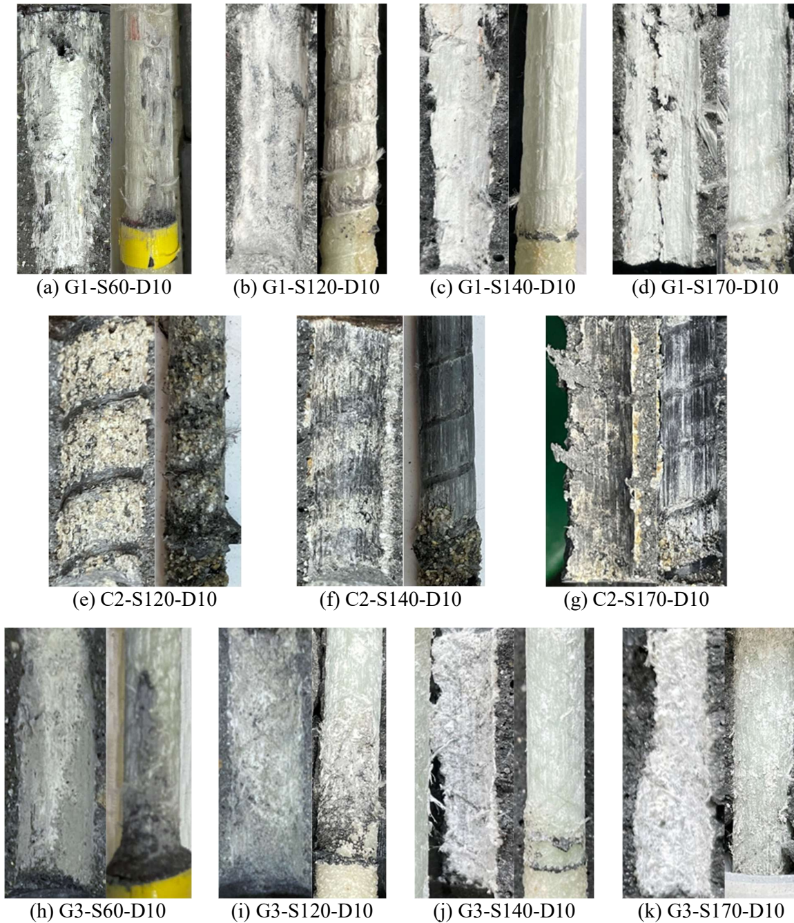
Figure 3.13. Typical debonding surfaces of FRP bars from three producers
