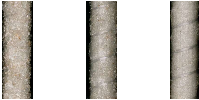
(a) densely sand-coated (b) moderately sand-coated (c) sparsely sand-coated
