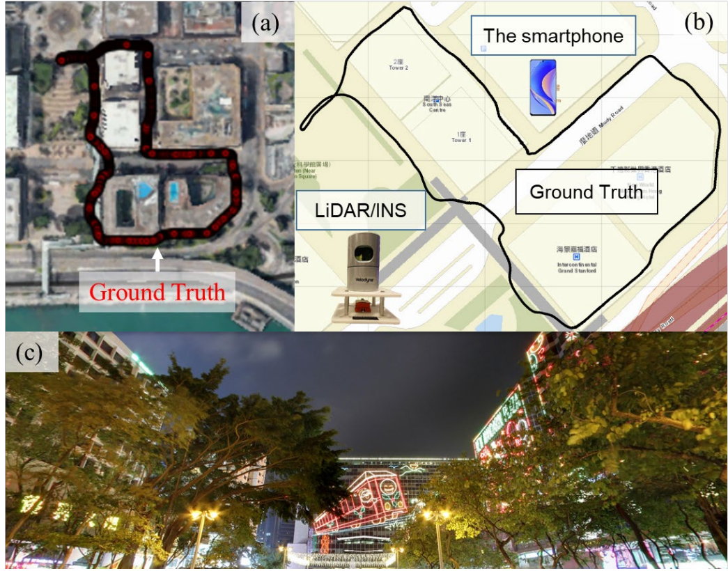
Fig. 3.5. The sensor setup of the mixed scenario. (a) image overview with GT from Google Earth. (b) the GT overview from OpenStreetMap. The LiDAR/INS system is used for generating the GT, HUAWEI P40 Pro smartphone is used for collecting the GNSS and IMU measurements. (c) Street-view of the scenario from Google Earth [85].
