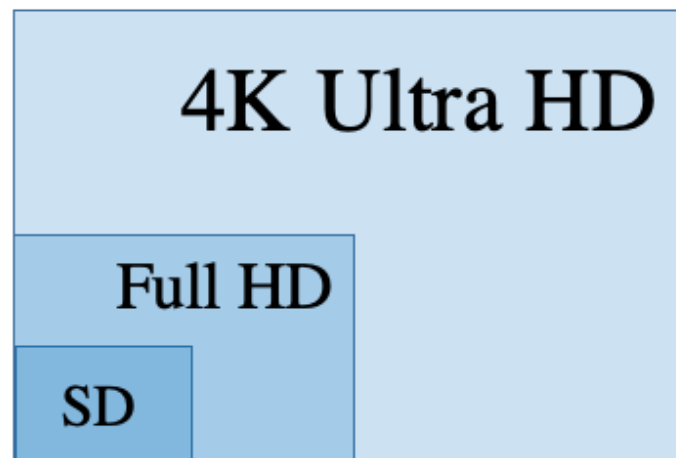
Figure 5.2: Standard Definition (SD): This is the lowest resolution, typically around 720x480 pixels. High Definition (HD): HD encompasses both 720p and 1080p resolutions, with 1080p also referred to as Full HD. Ultra High Definition (4K/UHD): 4K offers a resolution of 3840x2160 pixels, providing four times the pixel count of Full HD.
