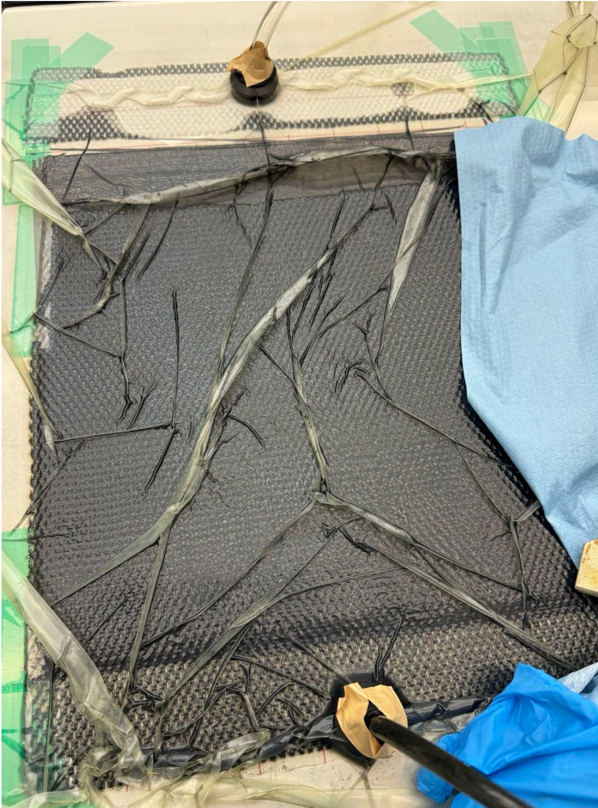
Figure 3.9 Resin permeated through the lay-up with resin infusion inlet and outlet silicone tube positioned at two sides
