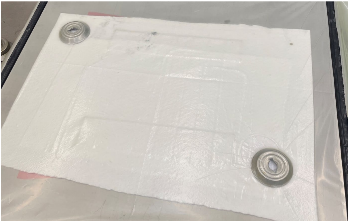
Figure 3.19 Two vacuum connector bases positioned at the corners of the metal plate in a diagonal manner
