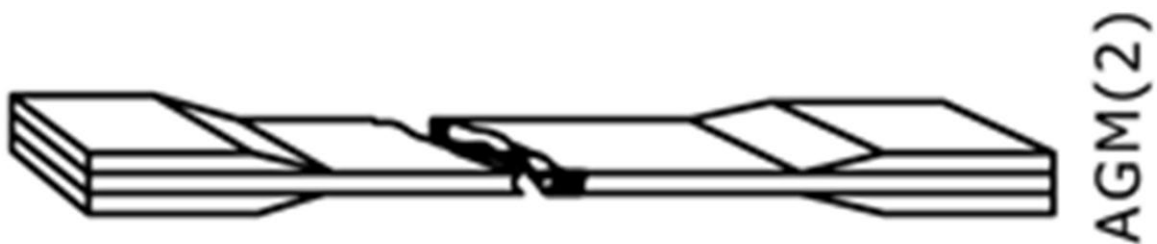
Figure 4.51 Specimen with failure mode - A G M (Angled type, Gage area, Middle location)
