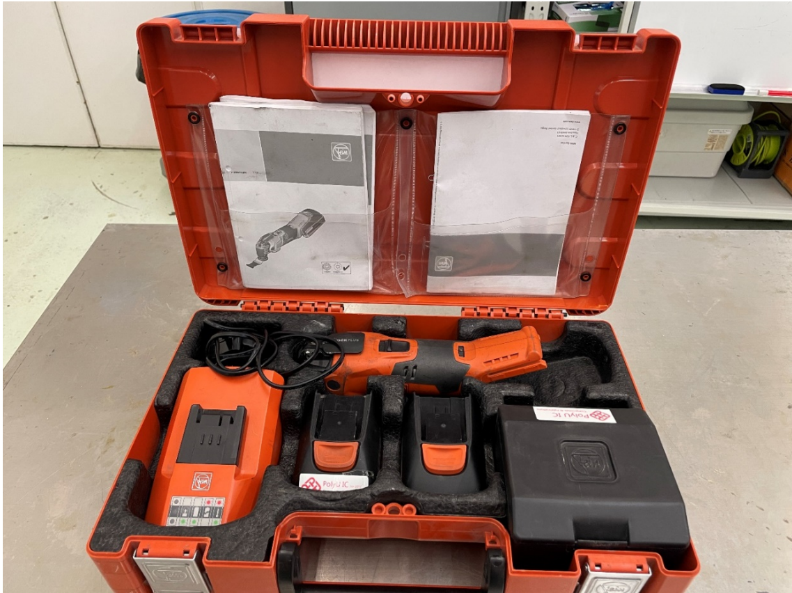
Figure 3.14 Sanding machine used to sand the materials surfaces
