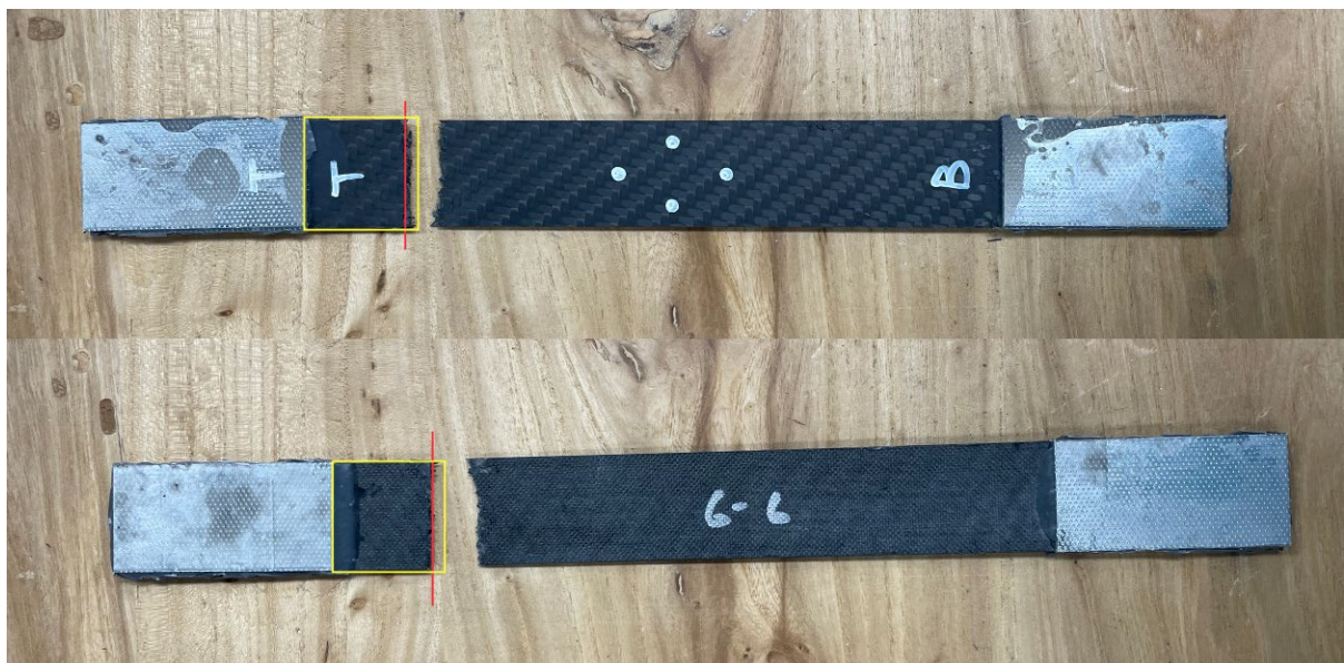
Figure 4.26 Specimen with failure mode - L W T (Lateral type, <1 Width from grip/tab area, Top location)
