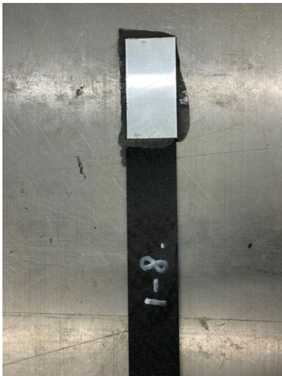
Figure 3.23 Separation of bonded specimens due to excessive adhesive
