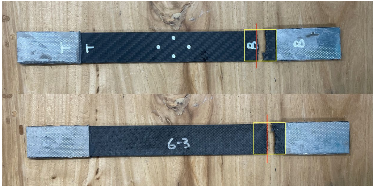
Figure 4.25 Specimen with failure mode - L W B (Lateral type, <1 Width from grip/tab area, Bottom location)
