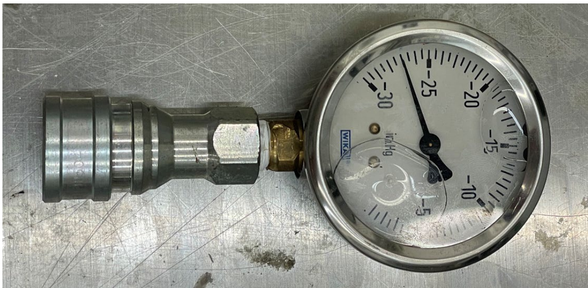
Figure 3.22 Pressure gauge in inHg
