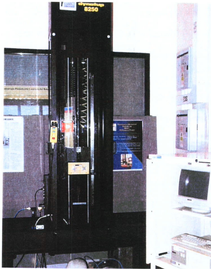
Figure 2.7 The Dynatup Drop Weight Impact Tester
