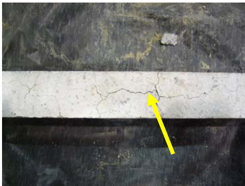
Figure 6.6.1. Extensive cracking on the surface of mortar bars.
