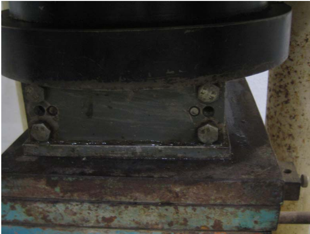
Figure 3.2.1a Water leak from the mould
