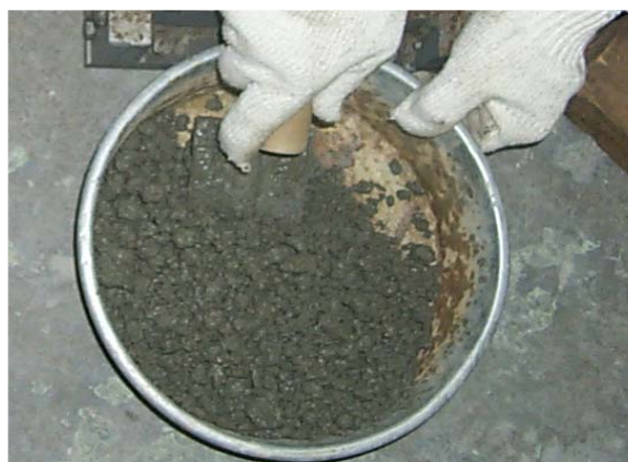
Figure 3.3.1.1 Dry mixture with suitable consistence
