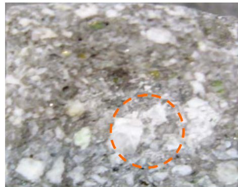
Figure 6.6.2. White particles/gel on glass cullet
