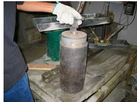
Figure 3.4.8.2 Place the load on the aggregates surface.
