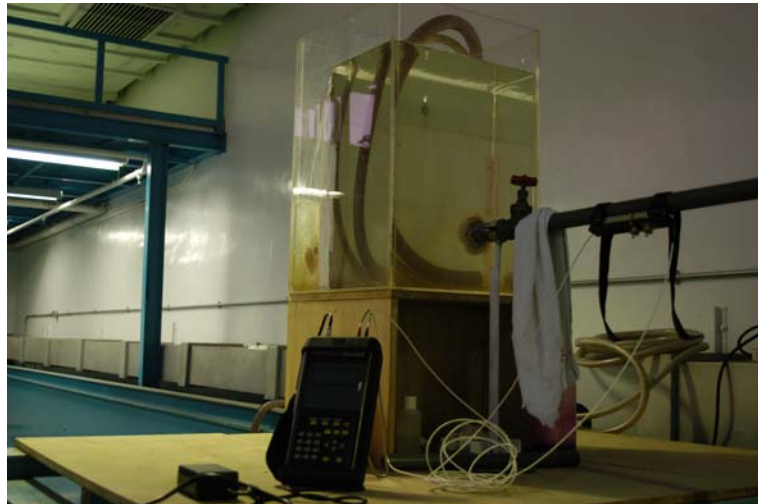
Photo 3.2. The constant head tank locates above the wave flume used in this study.
